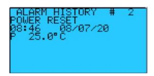
The ALARM HISTORY screen will display the last alarm that has occurred. The controller will store the last 100 alarms that have occurred. To view the Alarm History Log, press the ENT button to move the cursor to the alarm #. Using the UP and Down Arrow buttons scroll through the stored alarms
