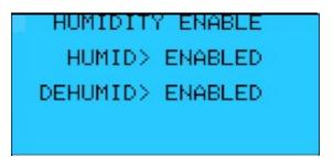
Note: This setting allows the user to enable or disable humidification or dehumidification if needed.
