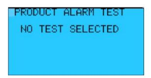
Press the ENT key to move the cursor to the NO TEST SELECTED data field. Use the Up or Down Arrow key to scroll through the tests. When the correct test is displayed press the ENT key to start the test. Press the ESC key to return to the System Status screen.
