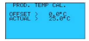
OFFSET: Allows calibration for the Product Temperature Sensor.
