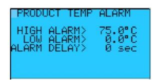
Factory Default Setting: High Alarm 75.0°C Factory Default Setting: Low Alarm 0.0°C Factory Default Setting: Alarm Delay 0 Sec
