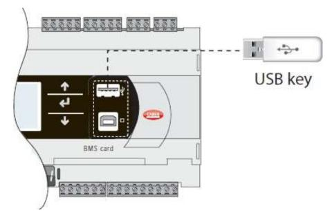
The USB port is intended for flash drives (USB key) only. Flash drive must be formatted as FAT32.
