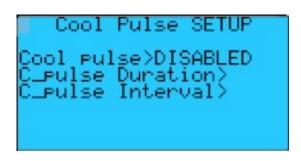
COOL PULSE ENABLE/DISABLE: Enables or disables the refrigeration cycling COOL PULSE DURATION: The length of the off time when cycling the refrigeration system COOL PULSE INTERVAL: The length of time between each on-off cycle when pulsing is enabled
