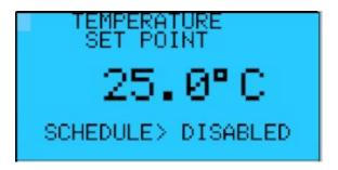
Note: If the schedule is enabled, the temperature will not be displayed on this screen and must be set through the ramp and soak schedule. To disable the ramp and soak schedule press the ENT key to move the cursor to the schedule field. Use the Up or Down Arrow key to disable the schedule. Press the ENT key and the cursor will move to the upper left-hand corner and the set point value will be visible. A full explanation of the ramp and soak schedule follows.
