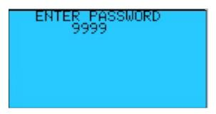
Press the Enter key to move the cursor to the four-digit password. Use the Up or Down Arrow key to increase or decrease the number. When the correct password is displayed press the Enter key to enter the password. If the correct password was entered the corresponding screen will be displayed. If a wrong password was entered "WRONG PASSWORD" will be displayed on the bottom line. The password can be re-entered or press the Escape key to return to the System Status screen.
