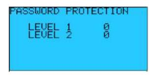
LEVEL 1: Password protection for the SET POINT and SENSOR TEST screens.
