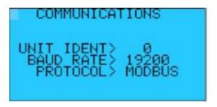
UNIT IDENT: Sets the unit identification for serial communications.
