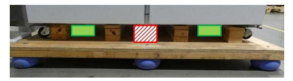
Remove foam/cardboard shipping supports from underneath plenum inside the chamber prior to powering on unit.
