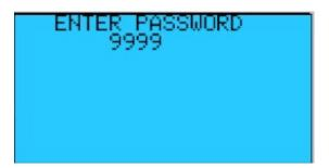
Press the Enter key to move the cursor to the four-digit password. Use the Up or Down Arrow key to increase or decrease the number. When the correct password is displayed press the Enter key to enter the password. If the correct password was entered the corresponding Set Points screen will be displayed. If a wrong password was entered "WRONG PASSWORD" will be displayed on the bottom line. The password can be re-entered or press the Escape key to return to the System Status screen.
