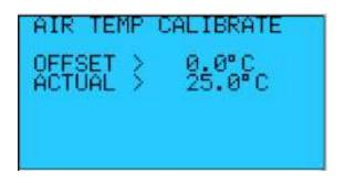
OFFSET: Allows calibration for the Air Temperature Sensor.
