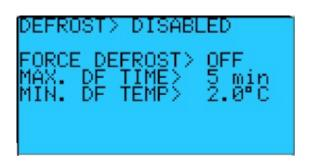
Factory Default Setting: FORCE DEFFOST > OFF Factory Default Setting: MAX. DF TIME > 5min Factory Default Setting: MIN. DF TEMP > 2.0°C
