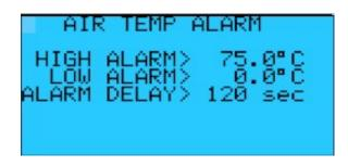
Factory Default Setting: High Alarm 75.0°C Factory Default Setting: Low Alarm 0.0°C Factory Default Setting: Alarm Delay 120 Sec
