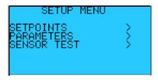
This screen allows access to the listed set up screens. Press the Enter to move the cursor to the desired field and press the Up or Down Arrow key to select the screens of each group.
